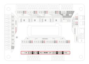
Power to the reader can be supplied using POE or a 12-28VDC external power source. DR40 has a maximum current rating of 791 mA at 12VDC, so should not be power directly by the DC20. Always check the power requirements of the door controller prior to installation. If PoE is not used, an Ethernet or Wi-Fi connection is required. Refer to Recommended Wire Type and Size table above for more wiring detail.
